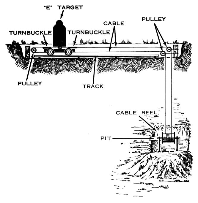
Figure 90. A moving target system.
