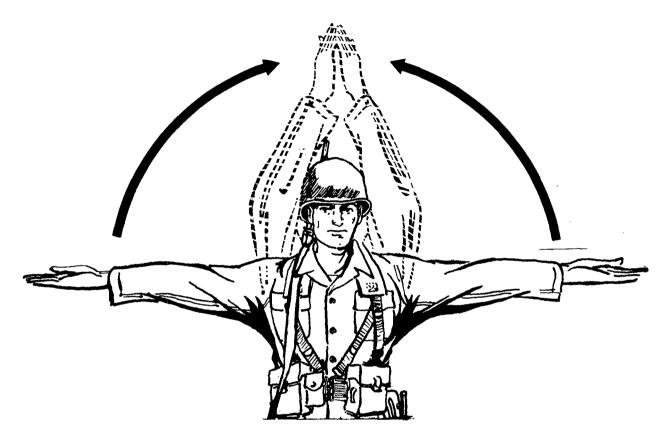
Figure 52. CLOSE UP. Start signal with both arms extended sideward horizontally, palms up, and bring palms together overhead momentarily. When repetition of this signal is necessary, return the arms to the starting position by moving them along the front of the body.
