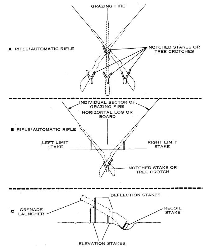
Figure 27. Field expedients for delivery of preplanned fires.
