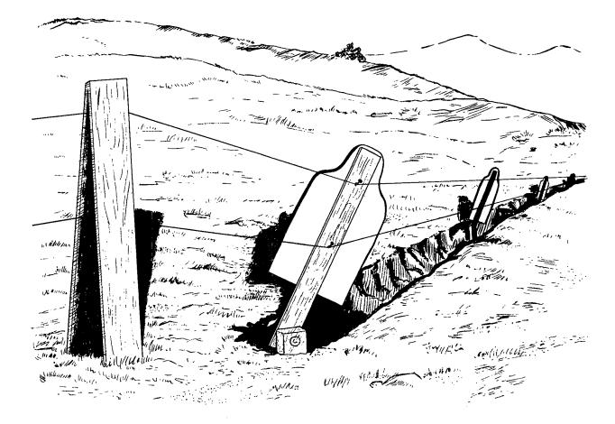
Figure 95. A method of raising linear targets.
