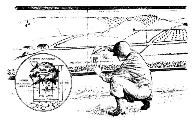
Figure 24. Template for marking point target scoring areas.
