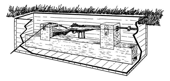
Figure 92. Rifle mount for installation in pit.
