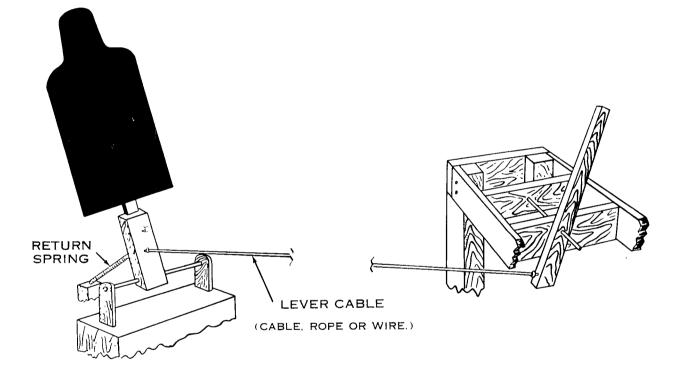
Figure 97. Manually operated pop-up target mechanism.
